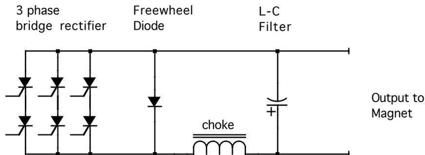
This arrangement is not ideal, however, because the capacitor is not protected directly by the diode. Any voltage that appears across the choke could appear as an added voltage across the capacitor. Depending on the exact L-C ratio and the slewing rates of the current, potentially damaging reverse voltages could appear across the capacitor.
