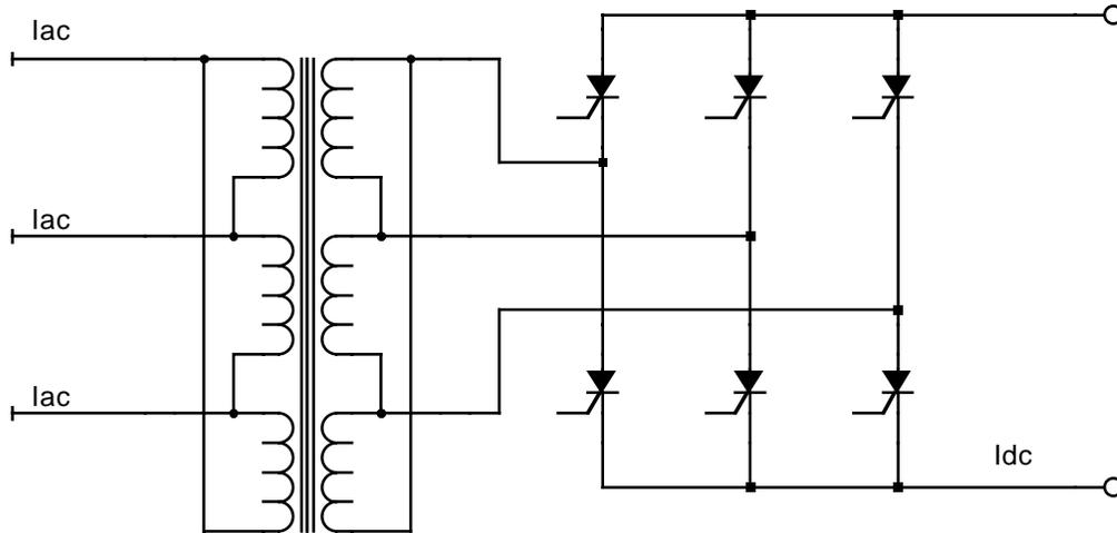
In conclusion, the power factor of a rectifier is variable over a wide range as the unit's output is varied. The maximum KVA occurs at full output power. As the output is decreased, the real power falls off as a function of the square of the current, yet the input KVA decreases linearly. This results in a power factor that can be estimated simply by knowing the output current of the power supply.
